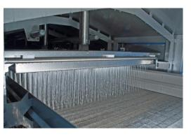
in maximum energy efficiency. A 30% to 40% reduction in steam consumption can be achieved compared to traditional steam blanching technologies because there is no escape of the steam when reheating the water.
