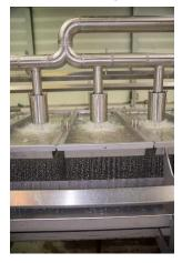
The OctoFrost™ IF Chiller has been designed to exceed all international regulations on food safety and hygiene. Every part of the chiller which comes in contact with the chilling water can be cleaned by CIP (Cleaning-In-Place).
